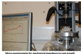
Micro-penetrometer for mechanical impedance to root growth
